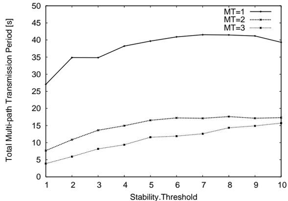
Fig. 7. The total multi-path transmission period versus *Stability.Threshold* and *Multi-path.Threshold*
