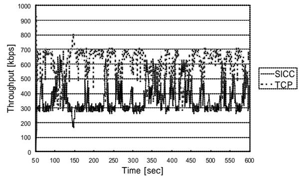
Fig 4 SICC and TCP throughput (RED)
