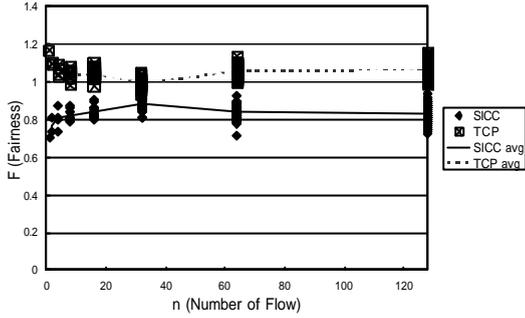
**Fig 5** TCP Fairness with n SICC and n TCP flows
