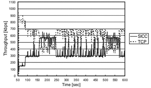
Fig 3 SICC and TCP throughput (DropTail)
