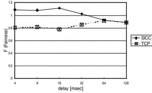
**Fig 7** TCP Fairness with SICC multicast and TCP
